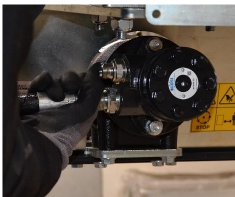
3 – 2 pcs. hydraulic hoses are mounted.
